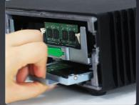
Hard disk is cableless and designed with a integration bracket for simple service
