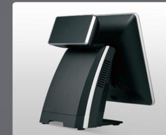
The integrated customer display can be turned and tilted for the best viewing angle.
