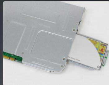
One step access to the SATA HDD or SSD for easy serviceability.
