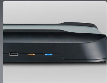
Power button, hard disk indicator and USB port is located in the front face for quick maintenance.
